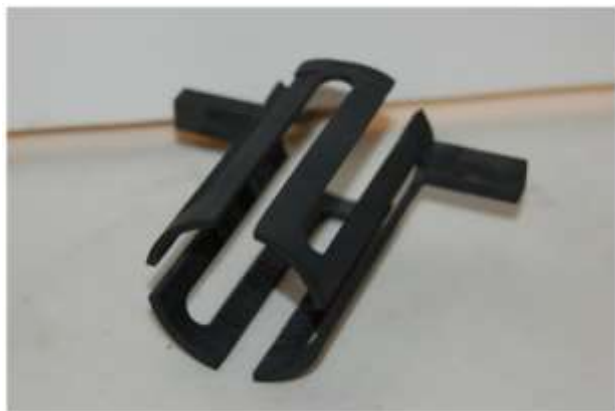
Figure 23 The graphite heater with 4 pseudo-coils [144].
