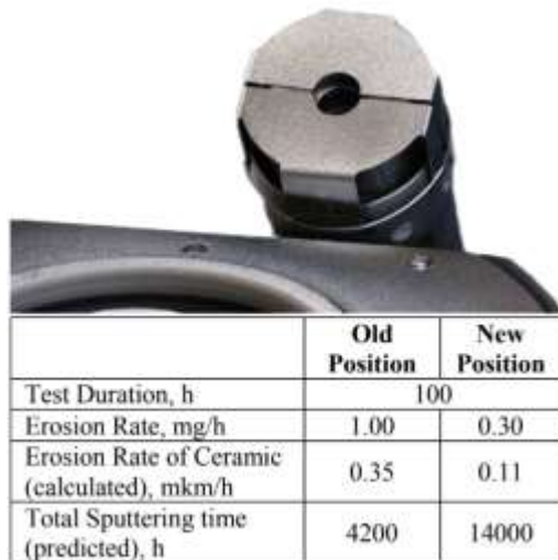
Figure 14 Half-cups erosion at the two positions [162].
