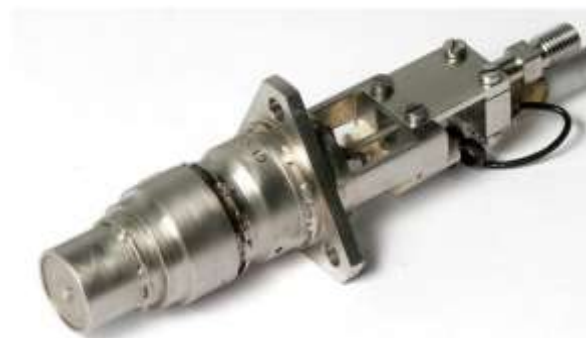
Figure 13 Photograph of the low-current hollow cathode [161].
