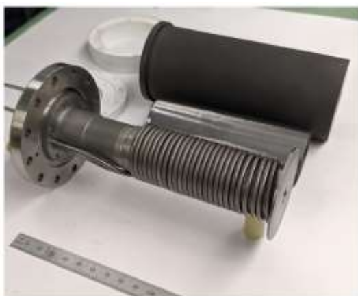
Figure 21 The enlarged orifice plate in the 500A hollow cathode [47, 79].
