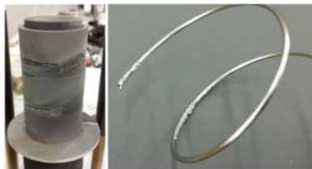
Figure 22 Photographs of the damaged boron nitride rings (left) and tungsten heater wire (right) [182].
