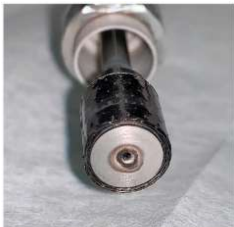
Figure 29 Post-test photograph of the cathode after keeper removal [194].
