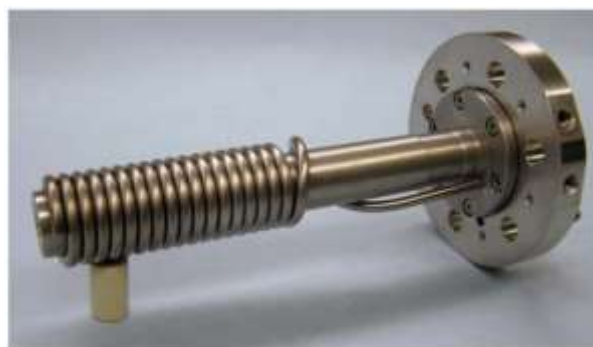
Figure 9 Tantalum-sheathed heater on the TDU cathode [150].
