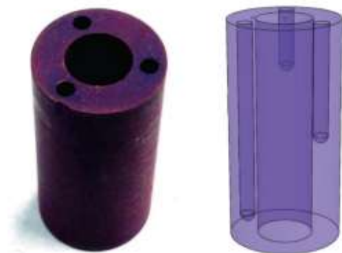
Figure 18 Three thermocouple wells drills in the \text{LaB}_6 insert [153].
